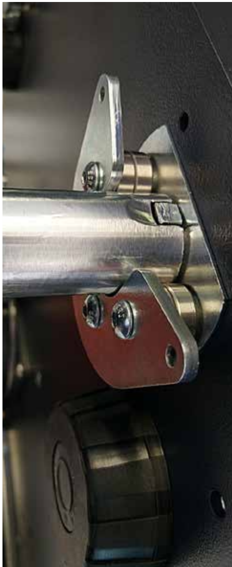
Drive via bolt-groove connection
