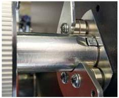
The drive bolt is inserted into the axle guide.
