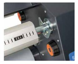
The driven axles are placed in the guide from above.
